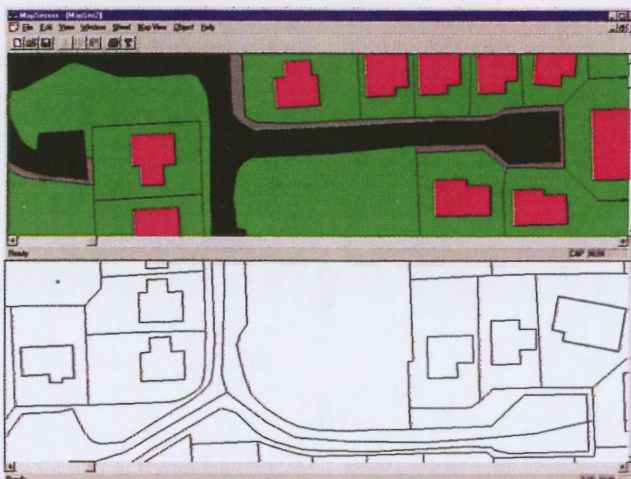
Before and after statistical analysis of map shapes. The upper window has been automatically colour-coded to indicate similar topographic objects.
