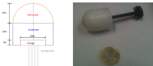
Fig. 5. A schematic diagram of the dielectric lens milled from HDPE (left). Photograph of the lens attached to the waveguide (right)
