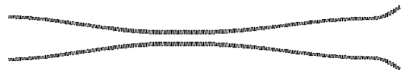
Fig. 3. General geometry of the PLANCK-HFI single-moded profiled flared cylindrically symmetric corrugated horn antennas.
