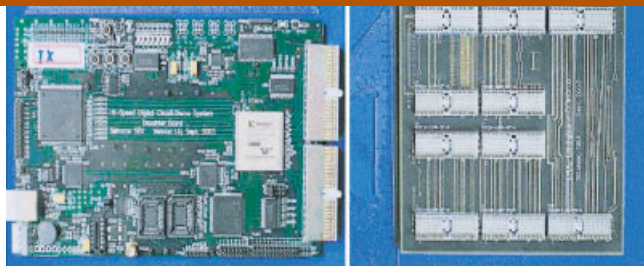
Figure 11 Photograph of the (a) daughter board and (b) backplane. [Color figure can be viewed in the online issue, which is available at www.interscience.wiley.com .]
