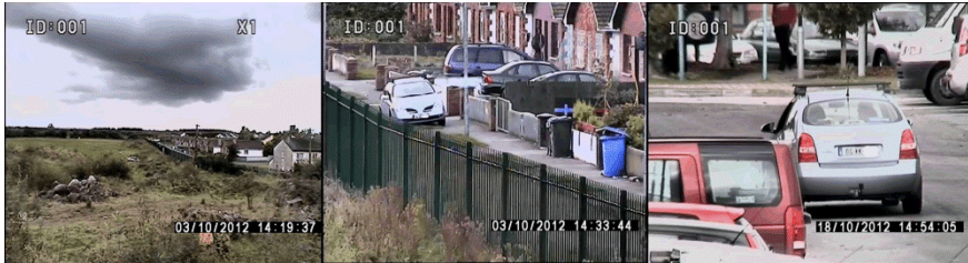
Figure 5: Long range 37X optical zoom camera images: (a) field of view with no zoom, (b) 25X zoom into area of interest, (c) 37X zoom with successful licence plate recognition over 180 meters.
