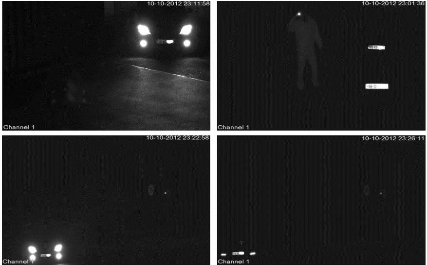
Figure 4: Examples of digital CCTV system images, from left to right and top to bottom: (a) camera + external illuminator licence plate recognition with the car situated 20m away and headlights on (b) camera + external illuminator licence plate recognition and action recognition in complete darkness; (c) camera + illuminator licence plate recognition car 33m away and headlights on (d) only camera licence plate recognition 33m away and back lights on.
