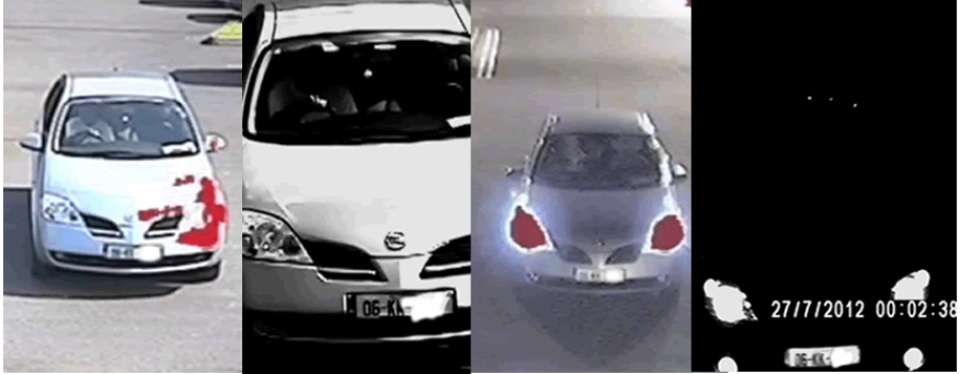
Figure 3: Examples of 600 TVL and LPR cameras images. From left to right: (a) 600 TVL camera in daylight, (b) LPR camera in daylight, (c) 600 TVL camera at night time, d) LPR camera at night time.
