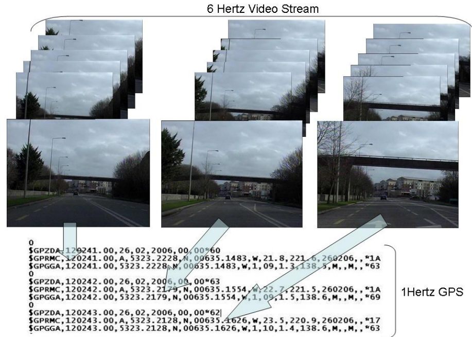
Fig. 1. This simple example of a partial Spatial Video stream depicts a minimal data set of video and GPS NMEA message relationships.
