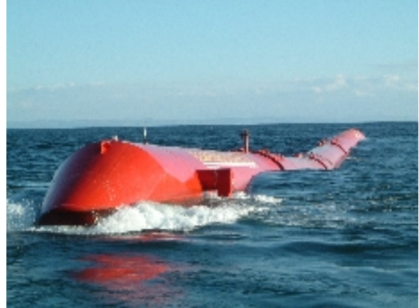
Fig. 7: The 'Pelamis' device [22]
