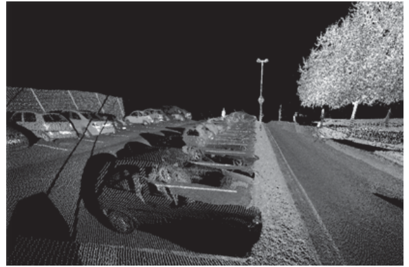
Figure 3: An example of a MMS Point Cloud
