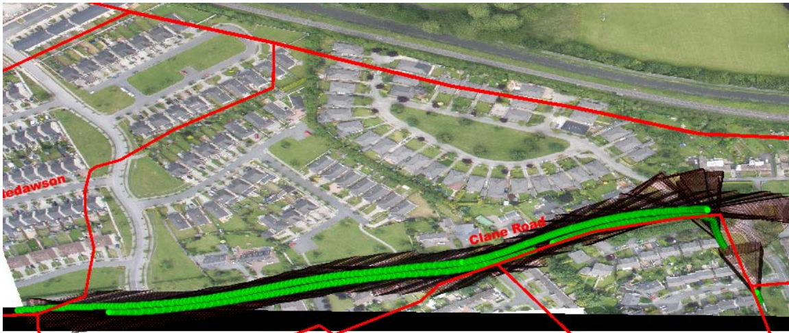
Figure 4. Viewpoint controlled polygon-in-view operation where the Clane Road query polygon is the search space. The result Viewpoints are shown as the green points with transparent red polygons. The geographical extent of each Viewpoint is either completely or more than 60% contained within the query region.
