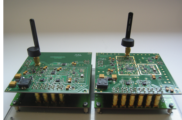
Figure 3 Low cost experimental SDR system from IMWS NUIM
