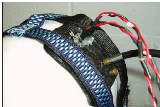
Figure 4 Rubber patch with embedded metal cylinders to support light sources and detector, Velcro straps hold the rubber patch in place
