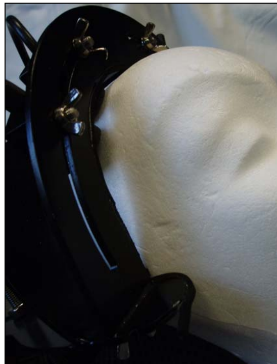
Figure 6 Optode holder for positioning light sources and detectors. It attaches to and slides along the supporting rails, securing optodes in place.
