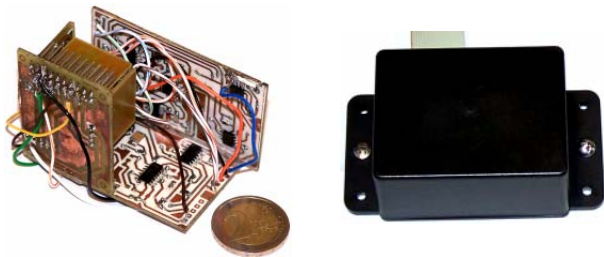
Figure 3 Sensor circuitry Using SMD & enclosed sensor.
