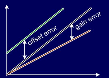
⇒ ADCs have individual transfer characteristics (gain, offset, DNL, INL)
