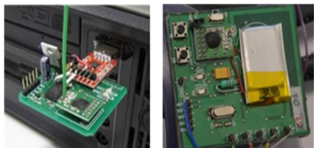
Gambar 5. Sistem haptic feedback; (a) pengirim; (b) penerima
