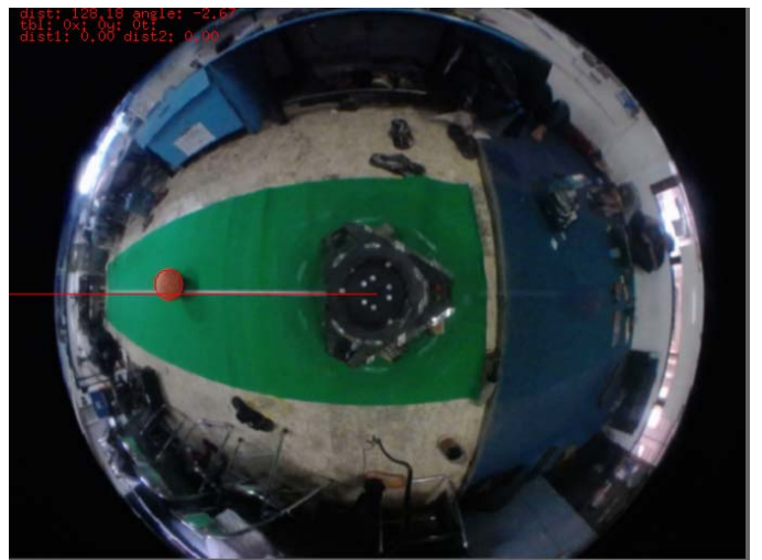
Fig. 4 Ball detection in 128 cm from the center of robot
