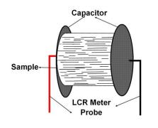
Fig. 6. Longitudinal position of the sample
