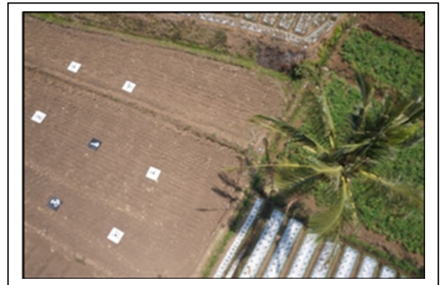
Fig. 6. Some of Ground control points on the field appear on the captured image
