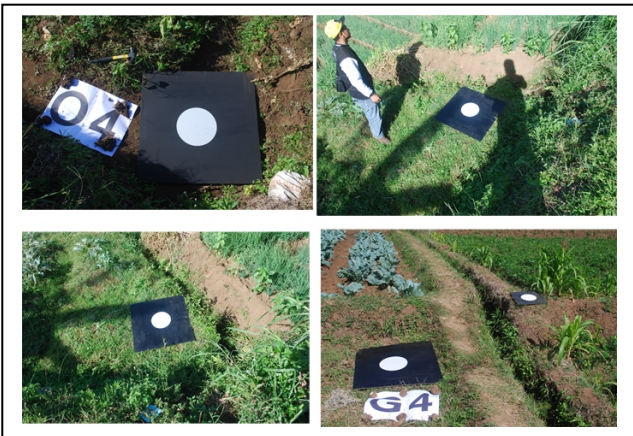
Fig. 3. Some of Ground control points on the field
