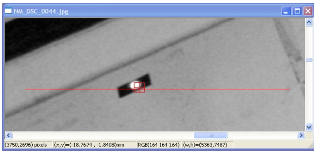
Fig. 6. Target patch on the normalized target image. An approximate conjugate point is resulted from normalized cross correlation matching method. A red line is an epipolar line.
