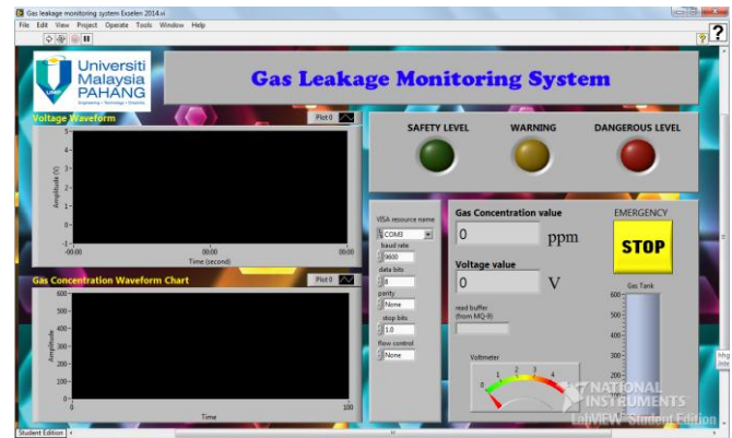
Fig. 3. The GUI of monitoring the gas leakage.
