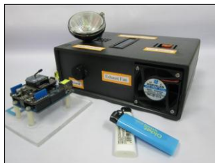
Fig. 14. Overall model configuration of the wireless gas leakage monitoring system with the gas detector.
