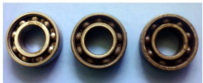
Fig.1. Normal, Damaged, and Badly Damaged Tested Bearings
