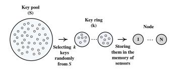
Figure 1. The process of key distribution.
