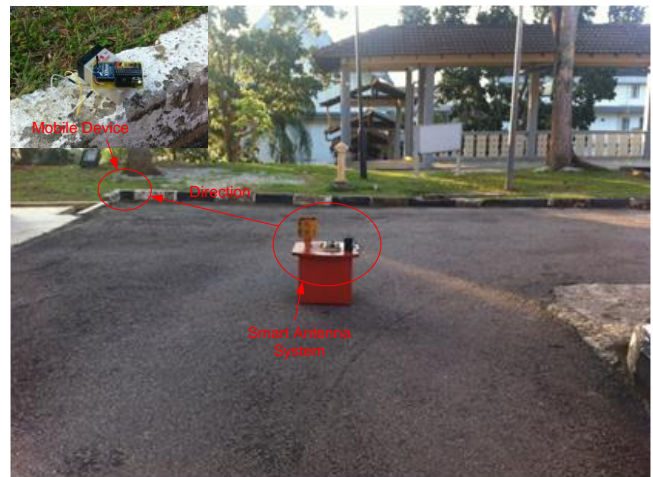
Fig. 9. Field testing of smart antenna system.
