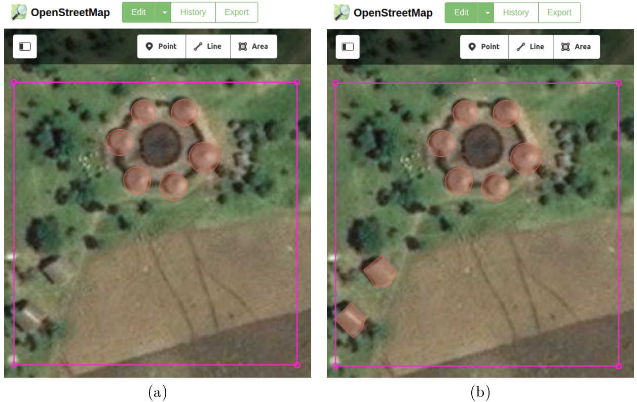
Figure 4.4: Gaphical User Interface of the iD editor for editing OpenStreetMap annotations: a) Tile (delimited by the bounding box in magenta) loaded for verification/correction of rural building annotations, b) OSM map after the annotation of two new buildings in the bottom left part of the tile.
