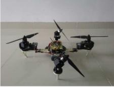
Fig. 6 Prototype of quad tiltrotor
