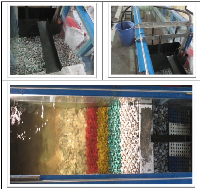
Fig 5. Overtopped water collecting chute and container
