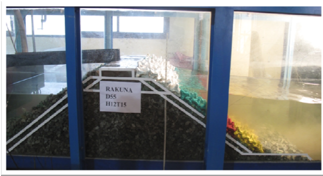
Fig 4. Model cross-section as built.
