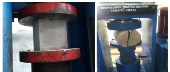
Fig. 1 Compression test (left) and splitting tensile test (right)
