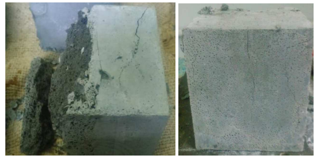
Fig. 4 Modes of failure (a) segregated LFC (b) normal LFC
