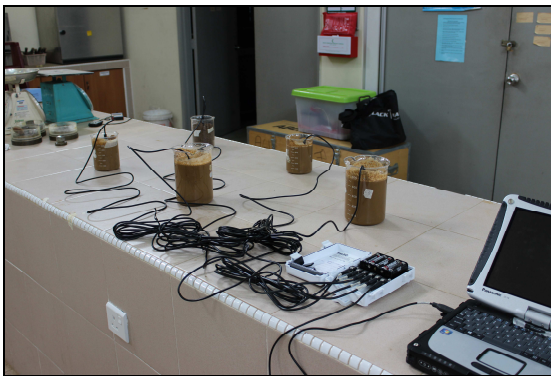
Fig. 2 5TE Soil moisture sensor calibration on laboratory
