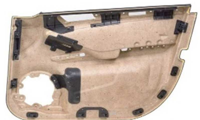
Fig. 7 Heated and molded mat into door panel
