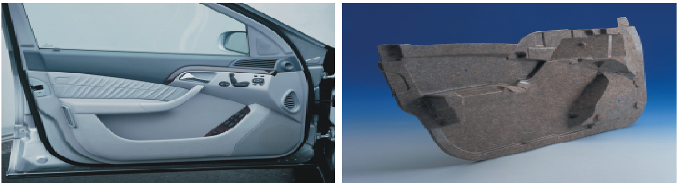
Fig. 5 Modern door inner trim panels are molded using mats of 60% natural fiber in a Baypreg® polyurethane resin (Courtesy of Bayer Polymers) [23]
