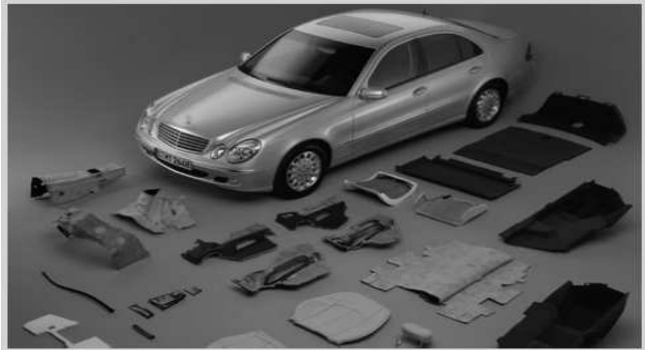
Fig. 4 Flax, hemp, sisal, wool and other natural fibers are used to make 50 Mercedes-Benz E-Class components [5]
