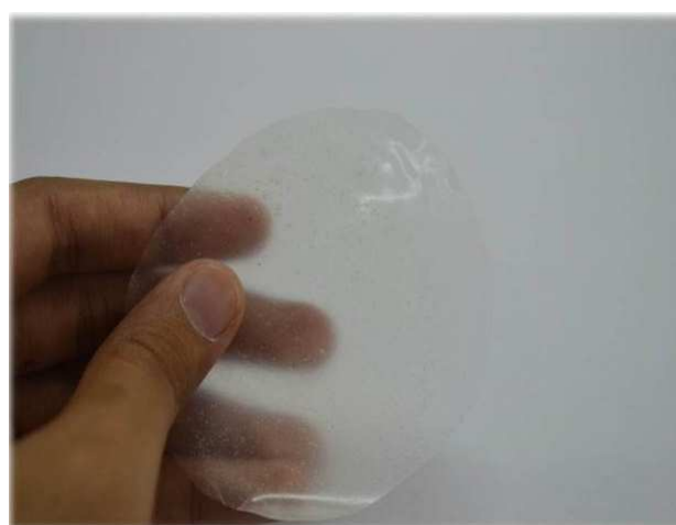
Fig. 1: A transparent edible plastic with a ratio of 20:20:10 wt% (gum Arabic: starch: glucose)
