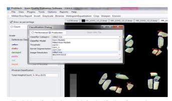
Fig. 7 Menu for selecting models for classification of current image
