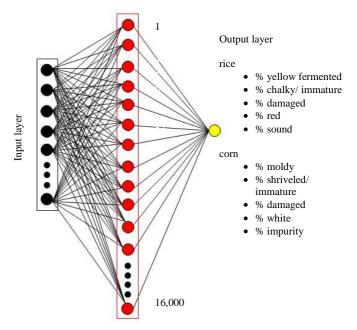
Fig. 2 A probabilistic neural network architecture
