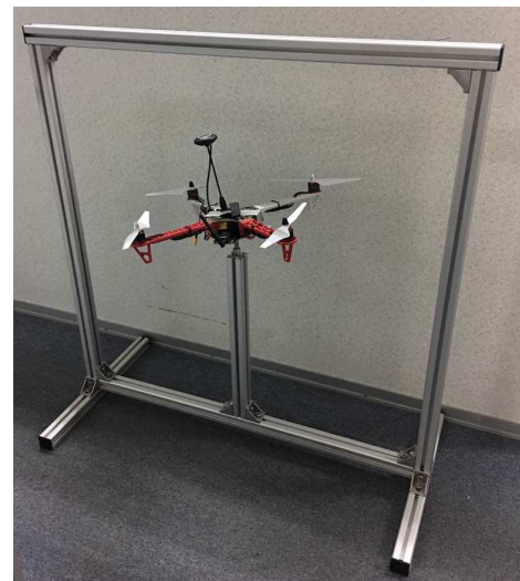
Fig. 2 x-configuration Laboratory Quadrotor UAV System
