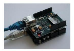
Fig.5 Arduino Duemilanove and Ethernet Shield
