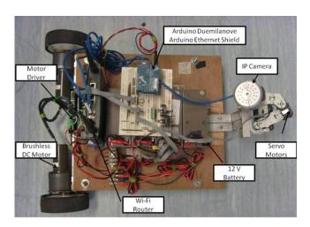
Fig. 3 Wi-Fi Surveillance Robot
