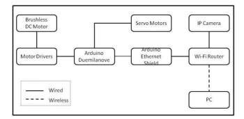
Fig.2 Functional Block Diagram of the Design
