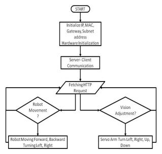
Fig. 8 Flow Chart of Embedded Web Server
