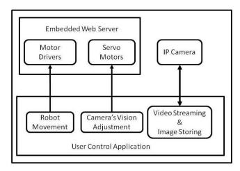
Fig. 9 Association of Embedded Web Server and User Control Application
