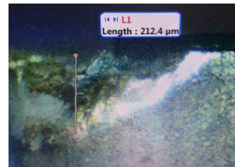
Fig. 9 Wear status and I-kaz coef. Values for Run 6 at DOC 0.4 mm
