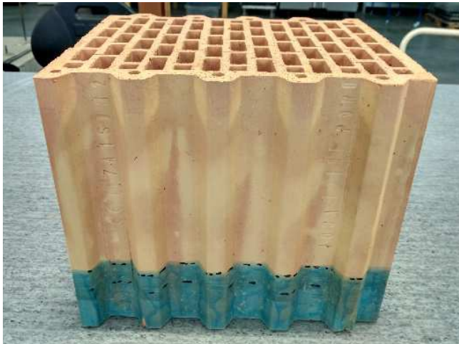
Fig. 10. Ceramic masonry block with the application of hydrophobic agent B (based on a silicon compound, nonylphenol, and ethoxylate) and pigment at a concentration of 1:40.
