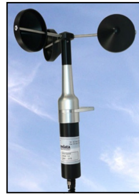
Fig. 1 Standard cup shape anemometer used for comparison in morphological chart [10]
