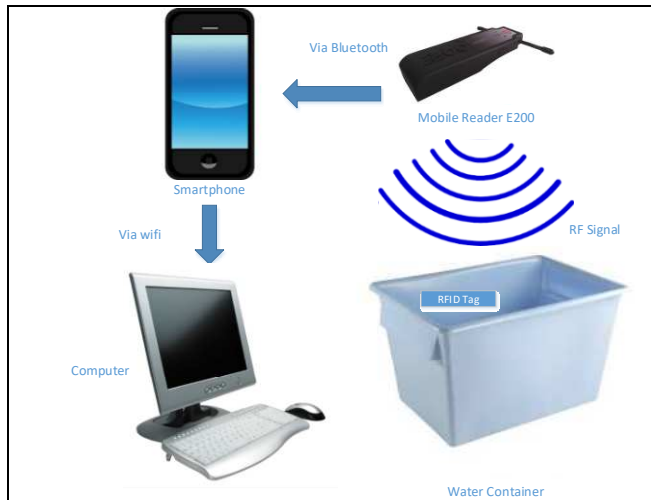
Fig. 4 Plastic container contains water and tag is read by the E200 reader
