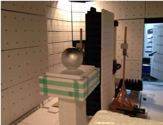
Fig. 9 Measurement scenario in a radio anechoic chamber performance against fluctuating targets, compared to without its implementation
