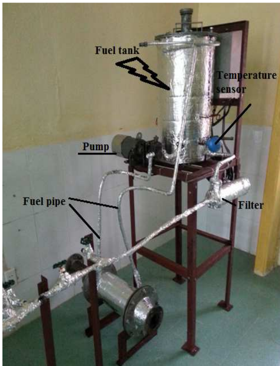
Fig. 1. A heating fuel supply system
