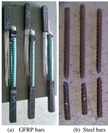
Fig. 11 Fracture Pattern of Reinforcement
