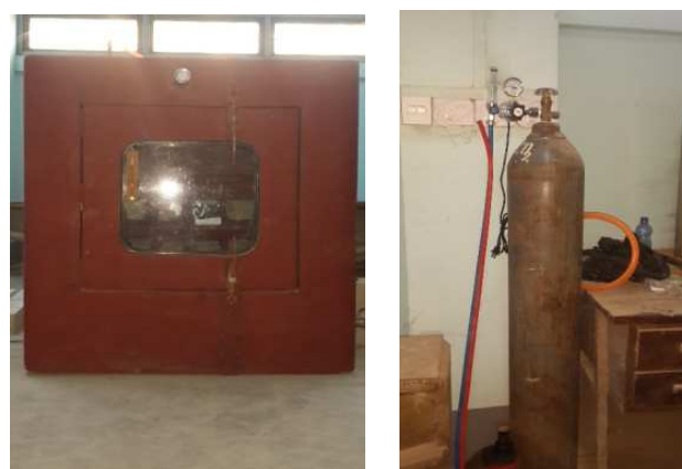
Fig 1. Carbonation Test Chamber
