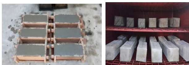
Fig 2. Preparation of Samples for Carbonation Testing
