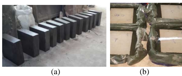
Fig 3. Preparation of Samples for Chloride Penetration Testing, (a) Slabs are Coated with Epoxy; (b) Slabs are Ponding with 3% NaCl Solution
