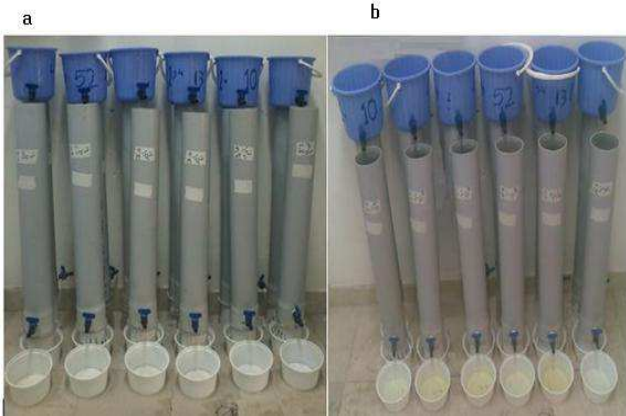
Fig. 3 A scheme of soil column and leaching soils. a) Continuous; and b) intermittent methods
