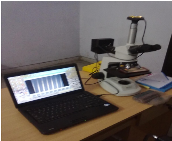
Fig. 4 KRUSS Metallurgical microscope used for measuring tool wears
