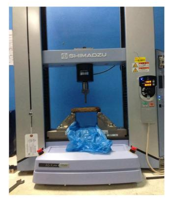
Fig. 5 Universal Testing Machine (Model: Shimadzu AGS-10kNXD) used to conduct 3 points flexural bending strength test in this research
