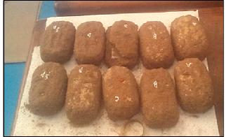
Fig. 1 Fabricated shell mould samples
