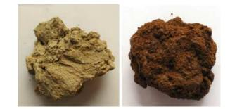
Fig. 4 Bentonite clays used as mould materials in this research, white bentonite (left) and red bentonite (right)
