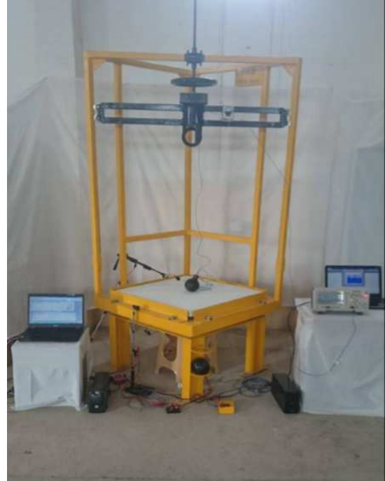
Fig. 2 Impact test apparatus with sensors
