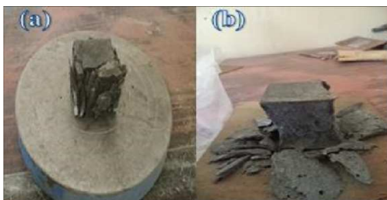
Fig. 4 Failure shape of the three RPC slabs' cubes
