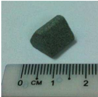
Fig. 6 Straight cut ceramic media
