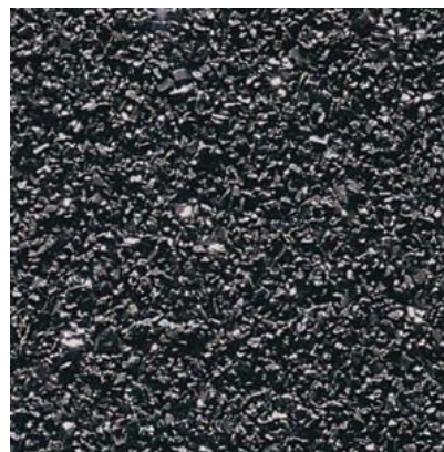
Fig. 3 Silicon Carbide Media
