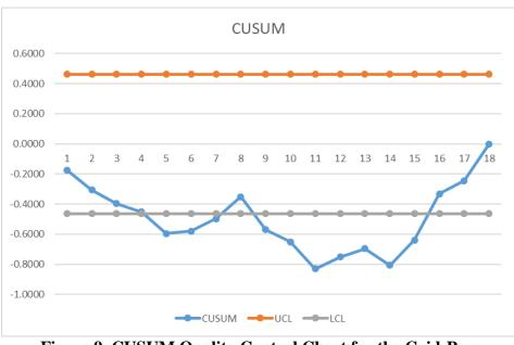
Figure 9. CUSUM Quality Control Chart for the Grid-Pan Temperature
