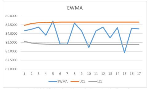
Figure 6. EWMA Quality Control Chart for the Sterilizer Temperature
