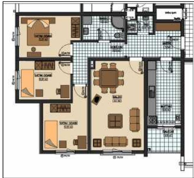
Figure 6: TOKI K2 Type Normal Floor Plan (Van Yüzüncü Yıl University General Directorate of Construction).
