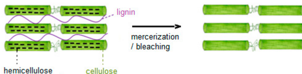
Figure 2. Representative diagram of the purification of natural fiber by alkaline peroxide.
