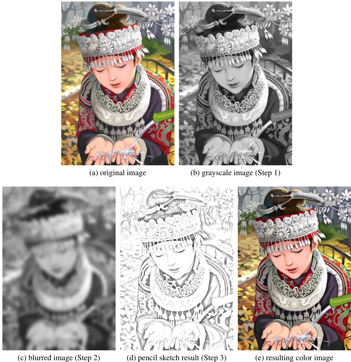
Figure 2.3: Results of the Pencil Sketch algorithm. (a) original image [78]; (b) grayscale image; (c) blurred image; (d) result of the division between images (b) and (c); (e) result of multiplying image (d) with Y-luma of image (a).
