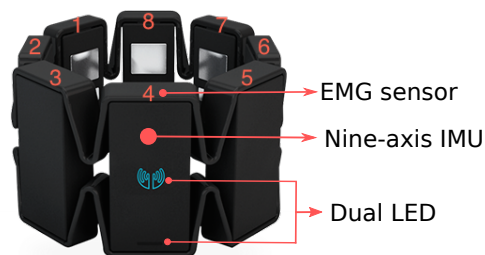
Figure 11 – Myo Armband Structure. Adapted from Thalmic Labs Inc. (2016a).
